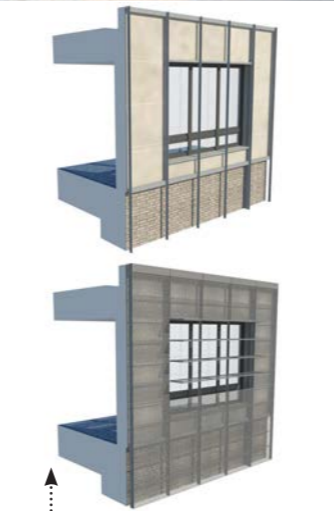
Royal Norwegian Embassy Beijing Contemporary design for a new extension to the Royal Norwegian Embassy in Beijing. The proposal was to add an additional floor to one of the buildings and create a new entrance space, to link the three Embassy buildings. The new structure is wrapped in a perforated zinc facade, which complements the brickwork of the existing compound and unifies the old and the new.
