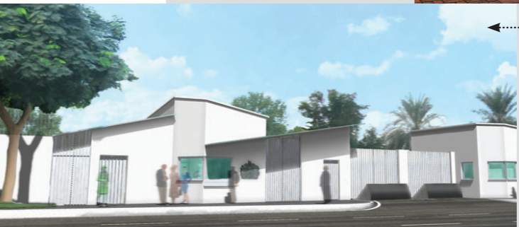
British Embassy Bahrain The building was conceived as two separate elements crossing at right angles with clerestory windows running along the length, providing light at high levels through the building. Brise soleil shading protects the building from glare and provides a comfortable working environment to the office space and public waiting area.
